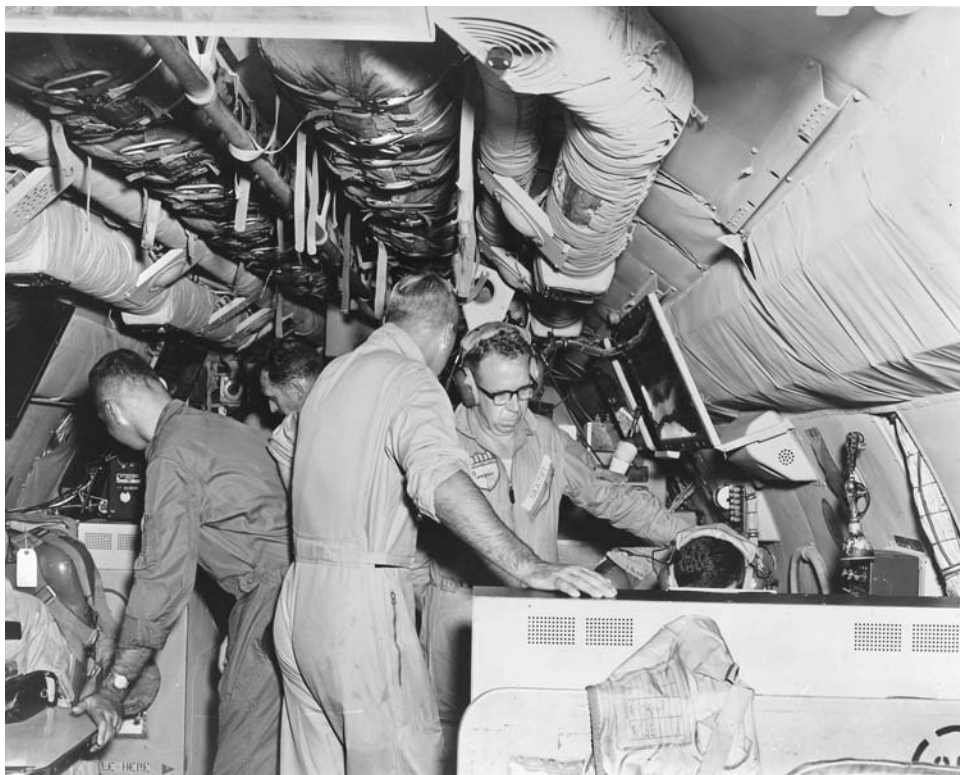
FIGURE 6.14. Interior of a Project Stormfury aircraft. Note the padding throughout the aircraft to prevent injuries during in-flight turbulence. NOAA Central Library.
