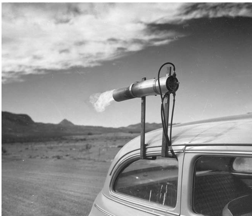
FIGURE 2.7. Mobile silver iodide generator mounted on an automobile for seeding experiments in New Mexico. From C. R. Holmes and William Hume II, “Final Research Report to the State of New Mexico Economic Development Commission Water Resources Development,” New Mexico Institute of Mining and Technology, September 1951.
