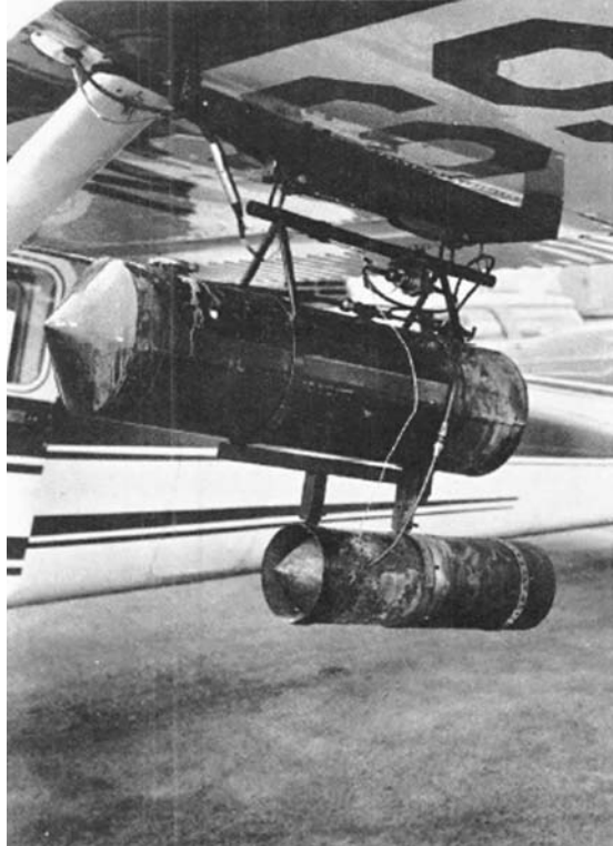
FIGURE 6.3. Project Skyfire airborne silver iodide generator. From Donald M. Fuquay, "Project Skyfire Progress Report, 1958–1960," Intermountain Forest and Range Experiment Station, Forest Service, USDA, Ogden, Utah, 1962.
