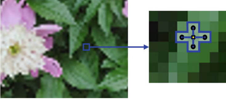
Fig. 4.4 An illustration of using spatial information of pixels to generate a hyperedge
