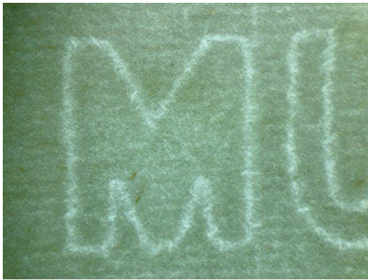
Fig. 5: Details of the structure of the sewn-on watermark letters in the paper.
