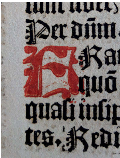
Fig. 5: Using magnification (8x), it is possible to see the printing sequence of colours, first red and then black. For a colour image, see Appendix, p. 442 of the print version.
