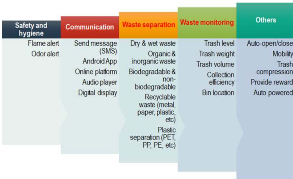
Figure 11.18 Key functions of smart trash bins.
