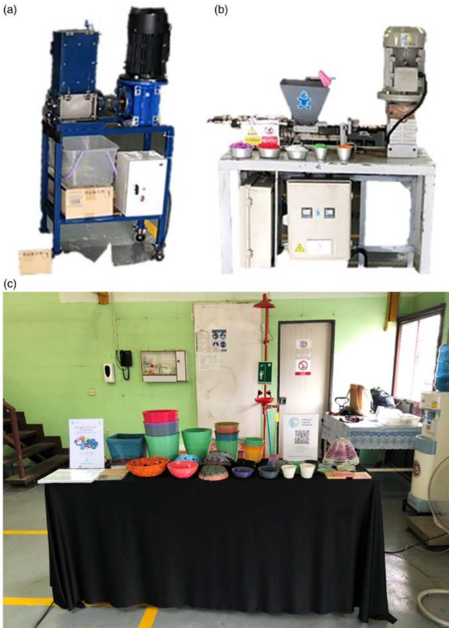
Figure 6.39 Precious Plastic Bangkok equipments and their products: (a) shredder machine; (b) extruder machine; (c) Precious Plastic Bangkok's products (Source: https://www.khaosodenglish.com/featured/2019/05/13/precious-plastic-recycling-bangkok-one-bottle-cap-at-a-time/ ).
