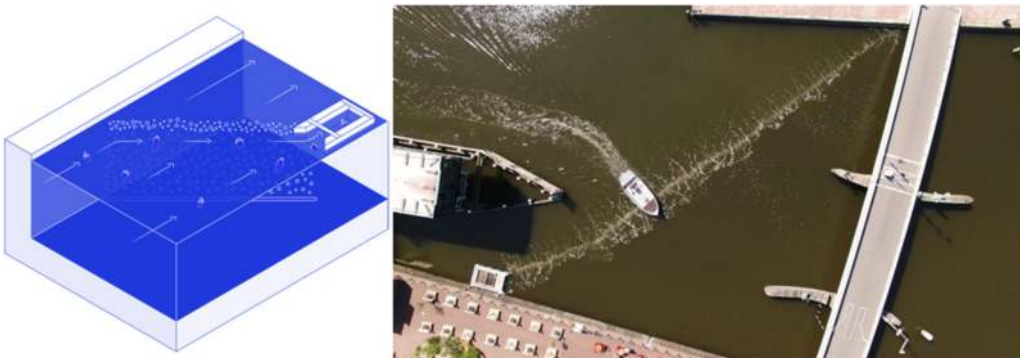
Figure 11.40 The Bubble Barrier system (The Great Babble Barriar, n.d.).
