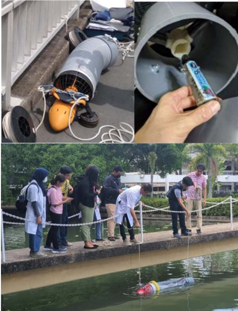
Figure 4.12 The albatross for microplastic sampling in the marine environment (Source: Abeynayaka et al., 2020 ).
