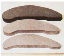
Above: Beryllium RF Antenna Tiles Production Sequence [2][3] Left: JET Reactor c.1982-83 Right: JET Reactor c.1990 with Be Belt Limiters Installed
