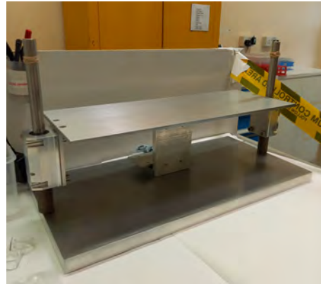
Pressure rig (test fixture) built at UKAEA and used in the study (the force gauge is not installed in this view). Design credit: Materion Corp., Ohio, USA Shown here with kind permission [7]
