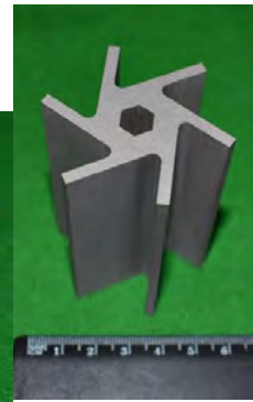
Six-bladed TiBe_{12} impeller \varnothing 50 \times 75 mm
