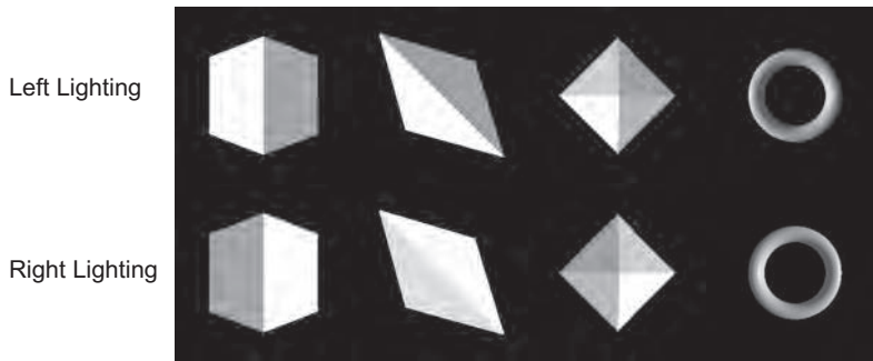
Fig. 2.76 Lighting invariance. VisNet was trained on a set of 3D objects (cube, tetrahedron, octahedron and torus) generated with OpenGL in which for training the objects had left lighting, and for testing the objects had right lighting. Just one view of each object is shown in the Figure, but for training and testing 180 views of each object separated by 1 deg were used. (After Rolls, E. T. and Stringer, S.M. (2007) Invariant visual object recognition: a model, with lighting invariance. Journal of Physiology - Paris 100: 43–62. © Elsevier Ltd.)
