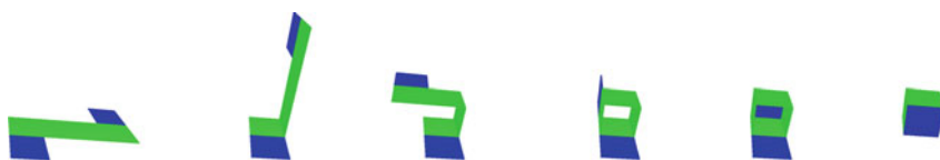
Fig. 13 Example of a reconfigurable assembly in the flexible tile assembly model. The glues between square tiles are flexible, similar to hinges, and allow the flat structure on the left to fold into the hollow box on the right
