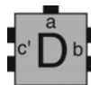
Fig. 1 Schematic depiction of an example (square) tile. Each glue (a.k.a. binding domain) is represented by the text label and black rectangle(s) on one side. The number of black rectangles corresponds to the integer-valued strength of the glue. The north (i.e., top) side has a strength 1 glue of type a , the east (i.e., right) side has a strength 2 glue of type b , the south (i.e., bottom) side has no glue (or the null glue), and the west (i.e., left) side has a strength 2 glue of type c' . The entire tile has the label D
