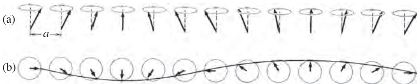
Figure 1.2. A spin wave on a line of spins. (a) The spins viewed in perspective. (b) Spins viewed from above, showing one wavelength. The wave is drawn through the ends of the spin vectors (after Kittel (1968)). From Introduction to Solid State Physics , 7th edition, by Charles Kittel, Copyright 1995 John Wiley & Sons Inc. Reprinted with permission of John Wiley & Sons Inc.
