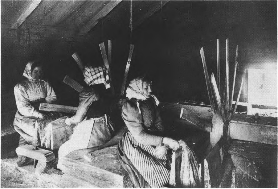
Women flax scutchers in a water-powered flax mill. Photo Hälsinglands Museum, Sweden.
