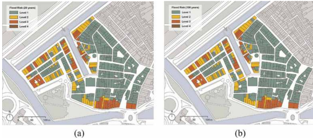
Figure 12. Spatial distribution of the flood risk results for 20 years (a) and 100 years (b).
