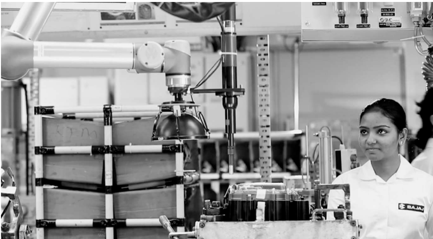
FIGURE 6.5 Cobot setup used by Bajaj Auto for automotive assembly tasks (adapted from UR, 2016c).
