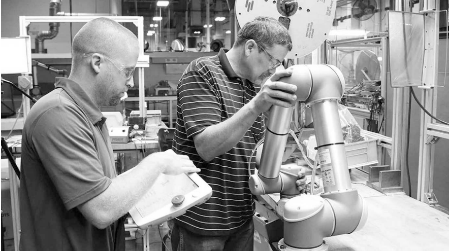
FIGURE 6.4 Use of cobot in low-volume, high-variant manufacturing line (adapted from UR, 2016a).
