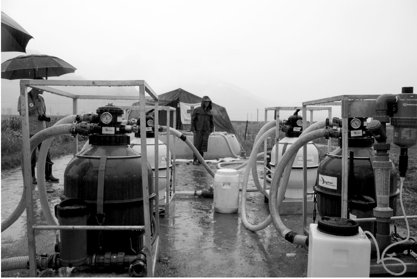
FIGURE 5.2. Emergency water units. Courtesy of Swedish Red Cross.
