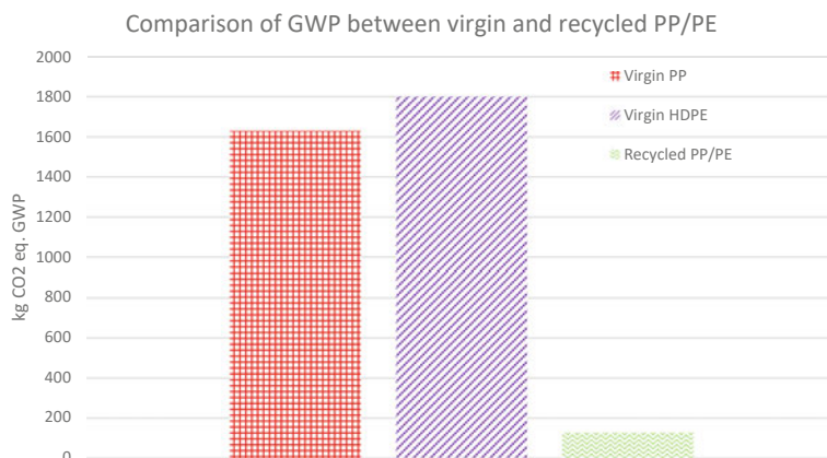
Fig. 7.4 Comparison of kg CO 2 equivalent emissions from the upstream and core production phases of virgin PP, virgin HDPE and recycled PP/PE granulate from fishing/aquaculture gear
