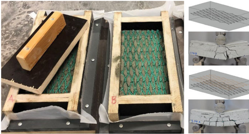
Fig. 12.9 Production of adobe bricks with one or two layers of fishing net reinforcement (Bertelsen et al. 2022)
