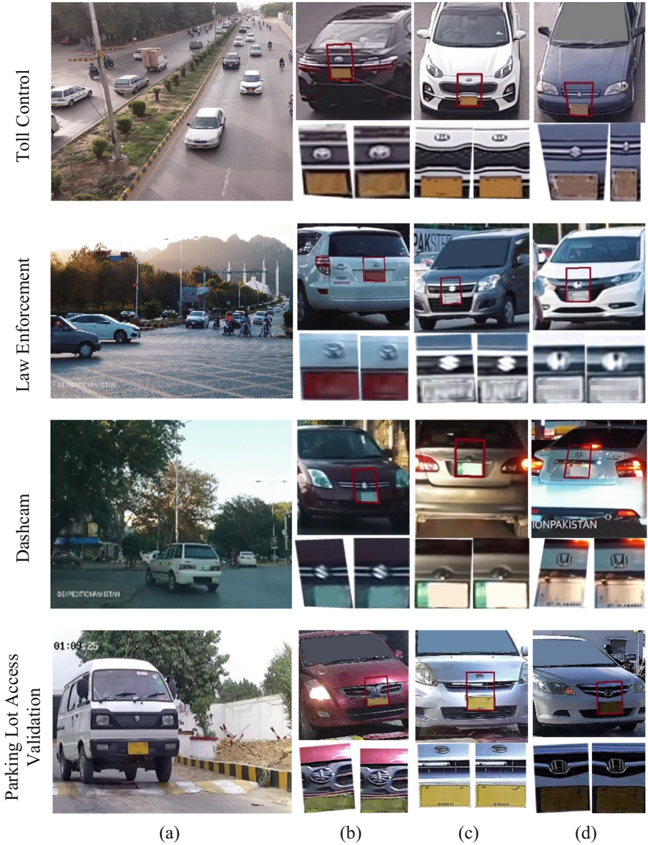
Fig. 4. (a) Single frame from each test case; (b)–(d) Individual vehicles in respective datasets of each test case along with their original logo containing ROIs and their respective unwrapped ROIs
