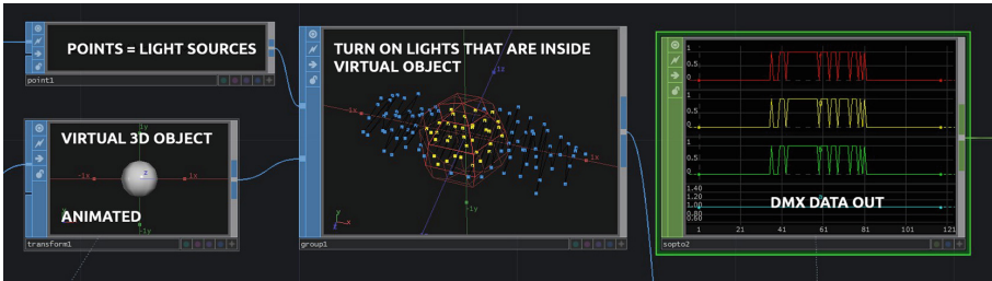
Fig. 1. Schema of light scene animation: Light sources represented as points in space collide with the animated virtual 3D object. Lights inside the object will be turned on.
