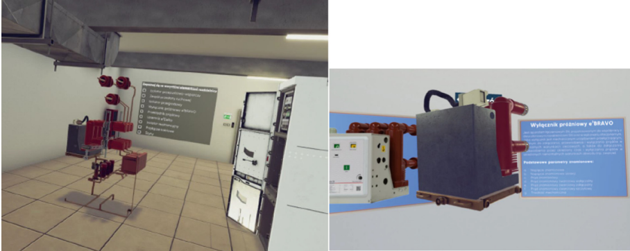
Fig. 4. Separated elements of the virtual switchgear (left) and the virtual model of the e2BRAVO circuit breaker (right).
