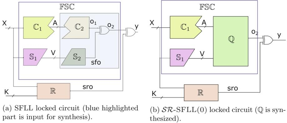
**Fig. 4.** Transformation of SFLL locked circuit to  $SR$ -SFLL(0) locked circuit. (Color figure online)
