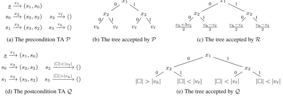
**Fig. 1.** Verification of a circuit  $C$  amplifying the amplitude of  $|00\rangle$  w.r.t. the specification  $\{\mathcal{P}, \varphi\} C \{\mathcal{Q}\}$  with  $\varphi: |v_h + 3v_l| > |2v_h|$ .  $\mathcal{R}$  is the TA obtained by executing  $\mathcal{P}$  on  $C$ .
