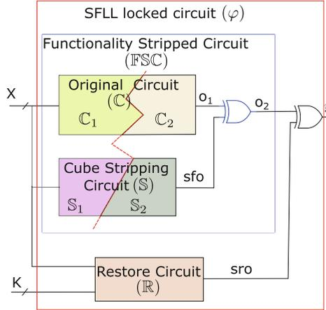
**Fig. 1.** SFLL-HD locked circuit ( $\varphi$ );  $\mathbb{C}$  is the (unprotected) original circuit. (Color figure online)
