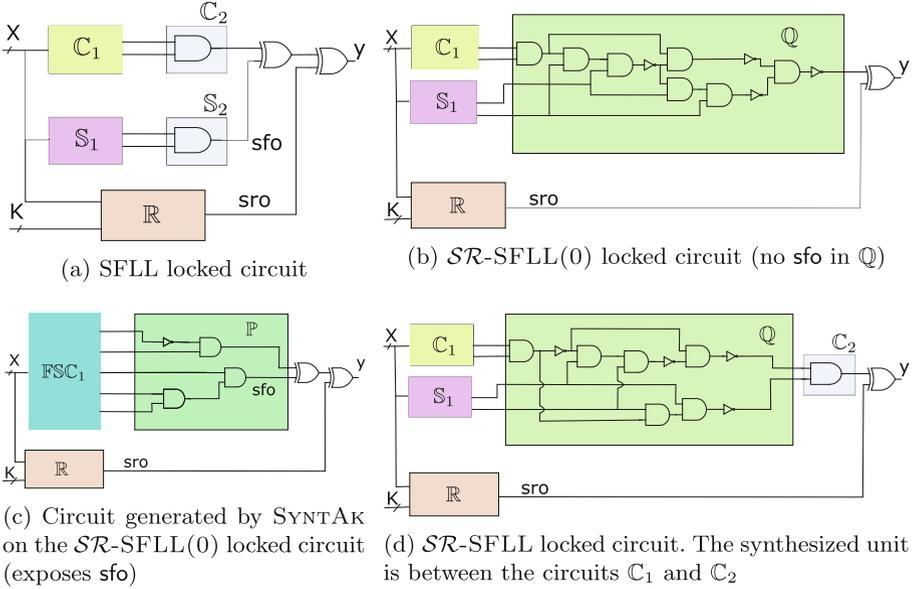
**Fig. 6.** Illustration of SFFL, SR-SFLL(0), and SR-SFLL locked circuits along with SYNTAK on SR-SFLL(0)
