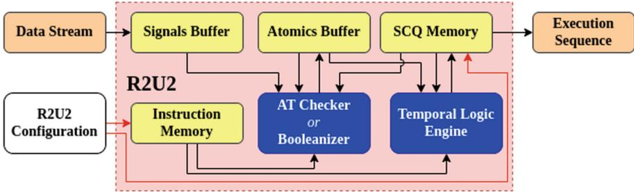
**Fig. 4.** Internal architecture of an R2U2 monitor. Orange boxes are streams of data, yellow boxes are memory arenas, and blue boxes are modules. Arrows entering and exiting blue boxes denote read and write relationships respectively. The red arrows denote relationships that are only active upon startup i.e., when R2U2 populates instruction memory and configures SCQ memory. (Color figure online)
