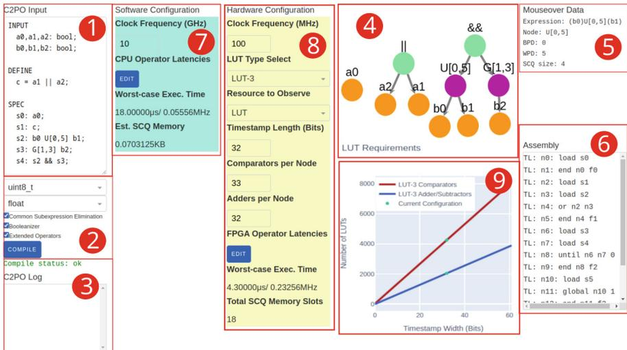
**Fig. 3.** R2U2 Configuration Explorer web application: 1) C2PO specification input; 2) C2PO options; 3) C2PO output; 4) AST visualization; 5) AST node data; 6) R2U2 instruction; 7) C engine speed and memory calculator; 8) FPGA speed and size calculator; 9) FPGA design size vs maximum timestamp value.
