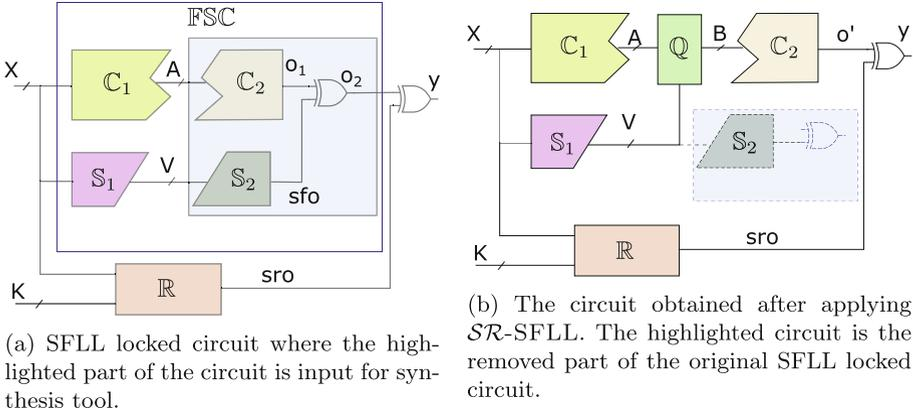
**Fig. 2.** Transformation of SFL locked circuit to  $\mathcal{SR}$ -SFLL locked circuit.
