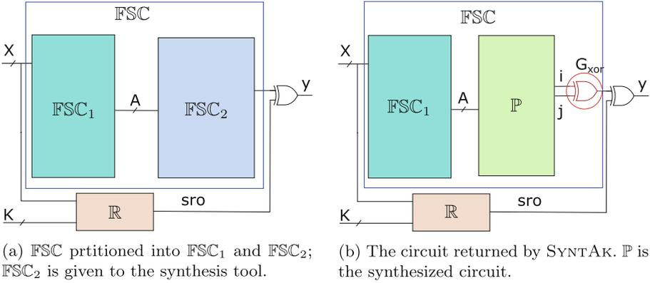
**Fig. 5.** SYNTAK on  $SR$ -SFLL(0) locked circuit.
