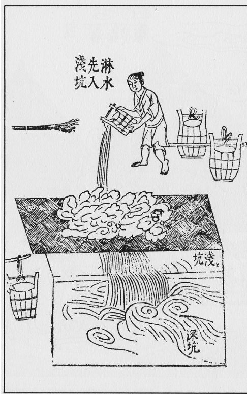
FIG. 5.2. This illustration represents a variation on salt-making techniques described by Lu Rong, as a worker pours briny water through a reed mat to drain into a pit below. From Sung Ying-hsing, T'ien-kung k'ai-wu: Chinese Technology in the Seventeenth Century , translated by E-tu Zen Sun and Shiou-chuan Sun (State College: Pennsylvania State University Press, 1966), 111.
