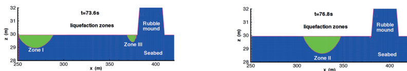
Figure 12.13 The three liquefaction zones in seabed under ocean wave at time t=73.6 s and t=76.8 s.
