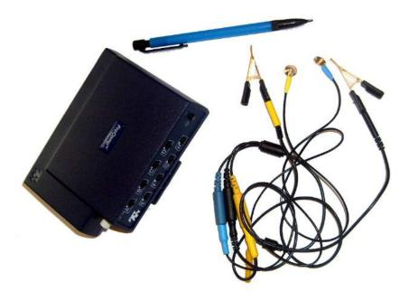
Figure 1: The ProComp Infiniti<sup>™</sup> EEG encoder by thought technologies.
