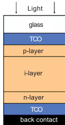
Figure 13: Structure of a typical amorphous silicon solar cell.
