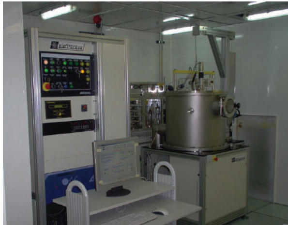
Figure 8: A commercial sputtering system for thin film deposition.
