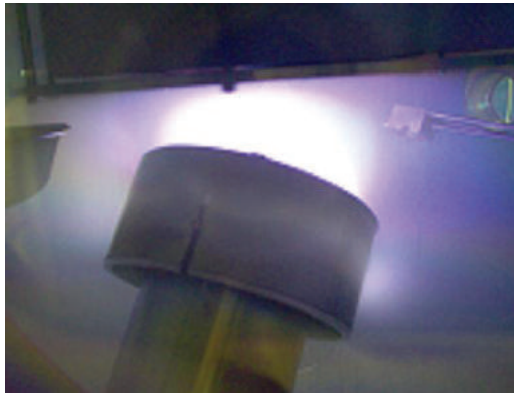
Figure 6: Sputtering cathode with plasma.
