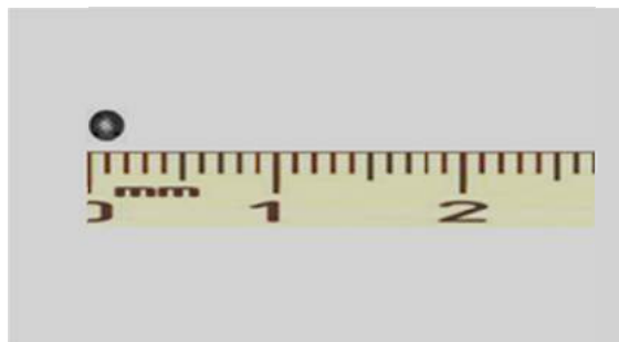
Figure 5: An iridium-platinum pellet measuring 1.7 mm in diameter with 2 holes drilled to form an X-Shaped cavity. The pellet was filled with ricin and encased in a waxy substance that melted at 37°C.
