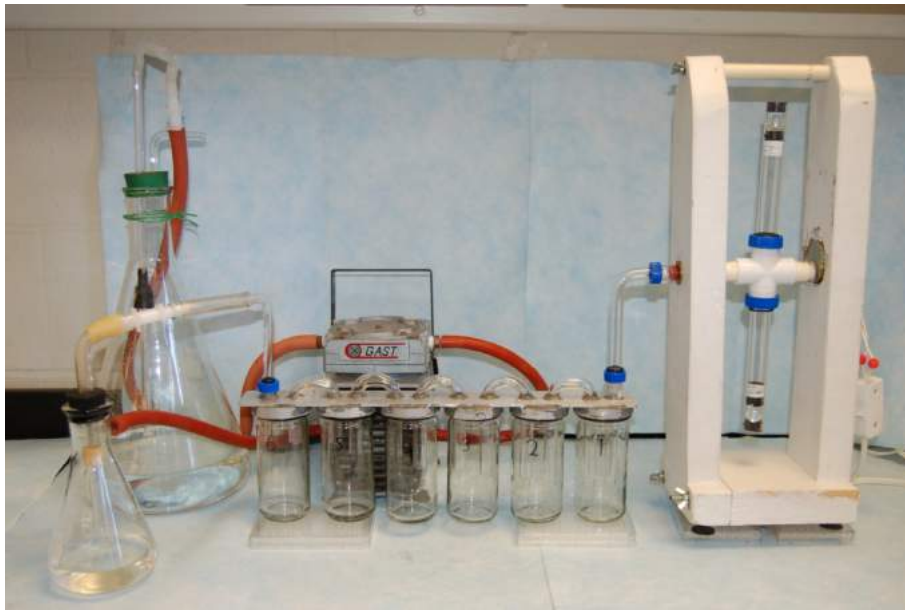
Figure 14: Dust generator rotating glass cylinders with ball valves and six dust trap bottles.
