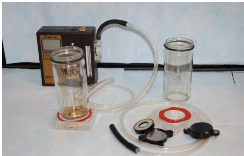
Figure 17: Personal Environmental Monitor air pump and PM10 and PM2.5 dust particle samplers. The modified dust collector bottles allow PM10 and PM2.5 dust collection from the fourth bottle in the dust collector.
