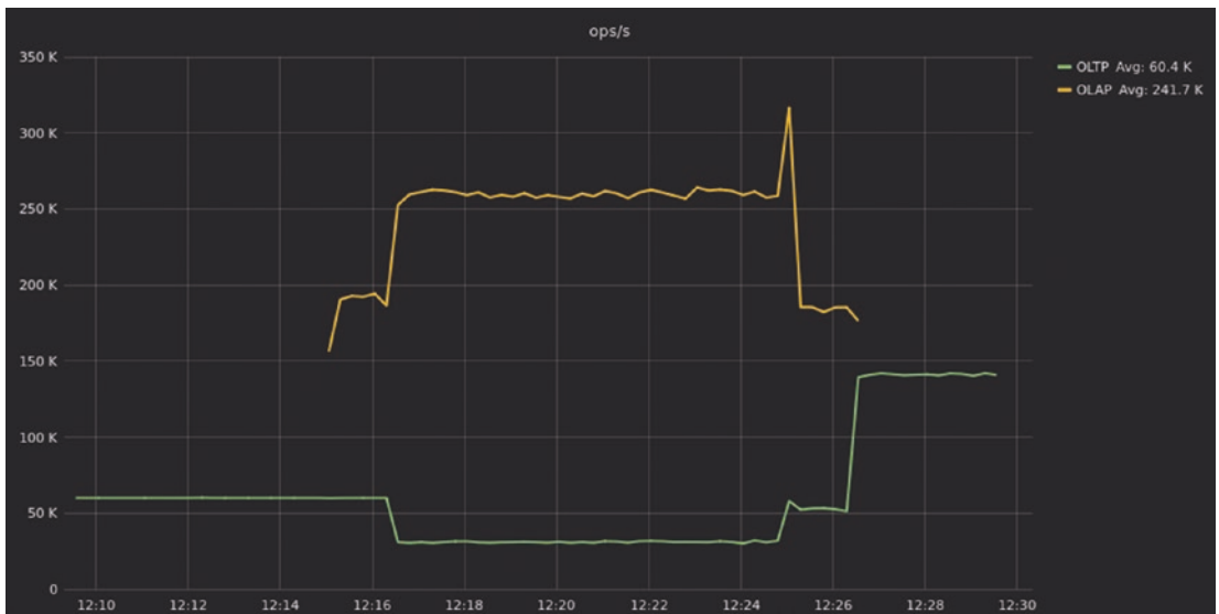
Figure 8-2. Comparative throughput results for OLTP and OLAP on the same cluster without workload prioritization enabled
