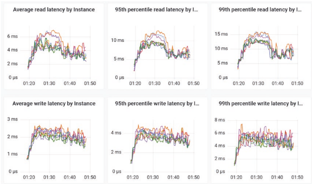
Figure 2-2. A sample database monitoring dashboard. Note the difference between average and P99 latencies
