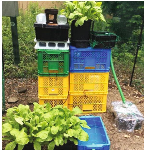
Fig. 4.1 Komatsuna cultivation system installed at the test site. Pots filled with noncontaminated soil were placed at heights of 30 cm and 120 cm above the ground. Basins filled with water were placed to collect fallout at the same heights as the pots
