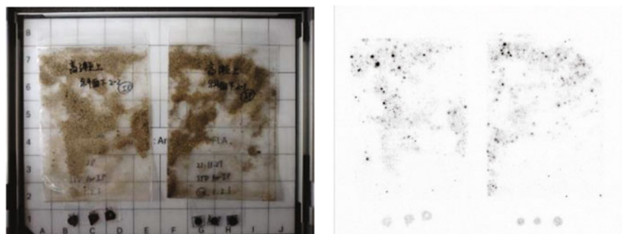
Fig. 19.2 Photograph and IP image of soil samples. Black dots indicate high Cs radioactivity
