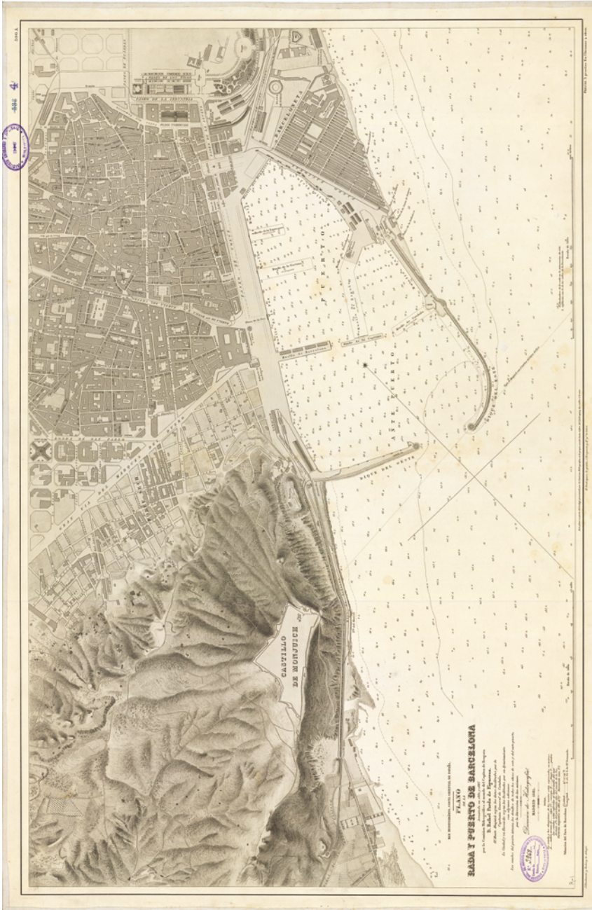
FIGURE 7.3 The port of Barcelona in 1882–83, when the first steps in its reform had already been carried out. The new quays and dikes and the demolition of the city's walls had moved the epicentre of the port westward SOURCE: DIRECCIÓN DE HIDROGRAFÍA (1885), PLANO DE LA RADA Y PUERTO DE BARCELONA: MAR MEDITERRÁNEO : COSTA ORIENTAL DE ESPAÑA, FILE SI-35-O-101, CARTOTECA DEL INSTITUTO GEOGRÁFICO NACIONAL
