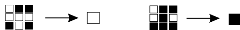
Fig. 1.6 Block-spin transformation in which we apply the majority rule to replace 3 \times 3 = 9 Ising spins by a single spin.
