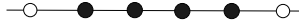
Fig. 8.7 A cluster of size four in one dimension. Occupied sites are drawn in black and unoccupied sites in white.
