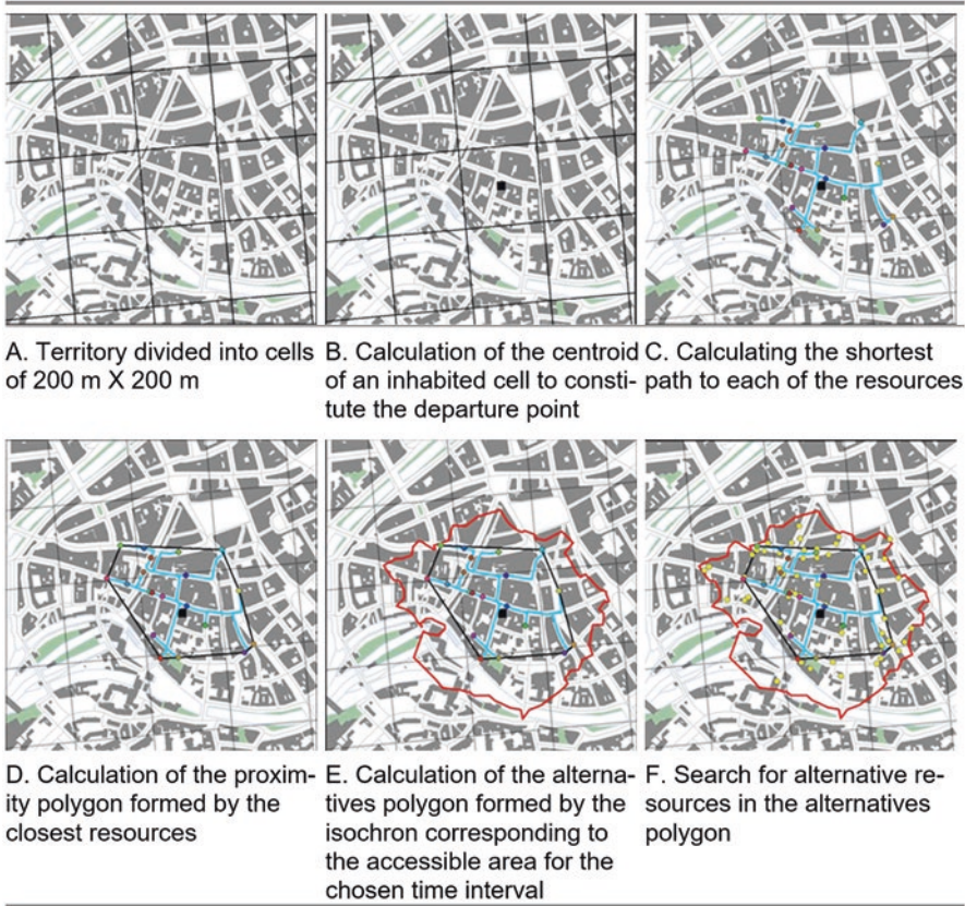
Fig. 4 Calculation of the proximity zone and the zone of alternatives within a 5-minute walking distance (the resources studied are common to both approaches, by isochrone and by path). (Source: Author, Hached, 2020). (a) Territory divided into cells of 200 m × 200 m. (b) Calculation of the centroid of an inhabited cell to constitute the departure point. (c) Calculating the shortest path to each of the resources. (d) Calculation of the proximity polygon formed by the closest resources. (e) Calculation of the alternatives polygon formed by the isochron corresponding to the accessible area for the chosen time interval. (f) Search for alternative resources in the alternatives polygon
