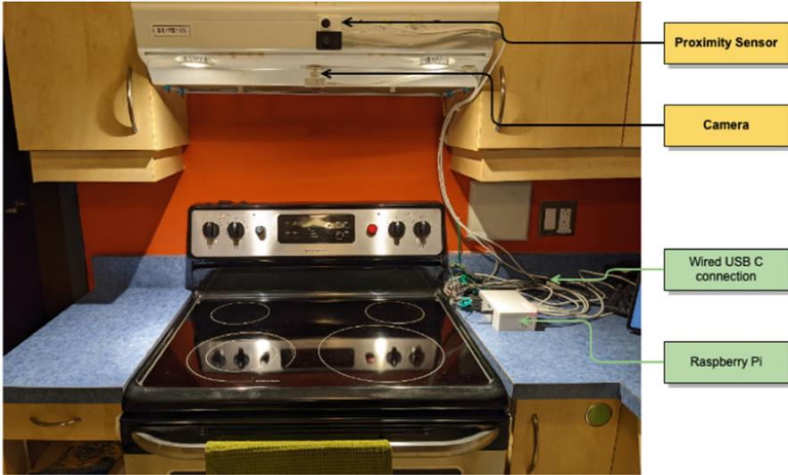
**Fig. 1.** Example of some sensors installed on the smart stove.
