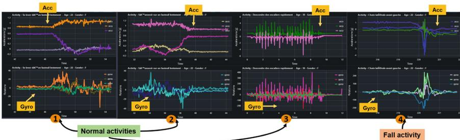
Fig. 3. Activities signal examples - Acc: accelerometer (acc\_x, acc\_y, acc\_z), Gyro: gyroscope (gyro\_x, gyro\_y, gyro\_z) - 3 Normal Activities (1, 2, 3) vs one Fall Activity (4)
