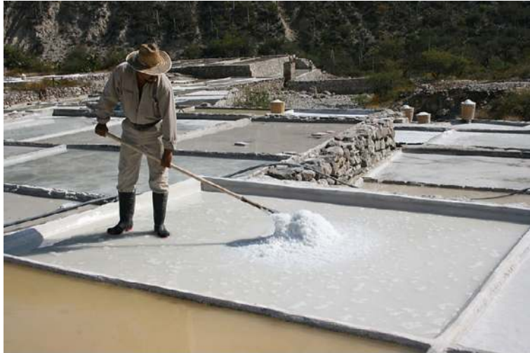
Figure 11. Zapotitlán Salinas, Puebla. Picking up the first salt in the center of the pond in November 2007. The baskets for drying the salt can be seen in the background (Photo by B. Castellón).
