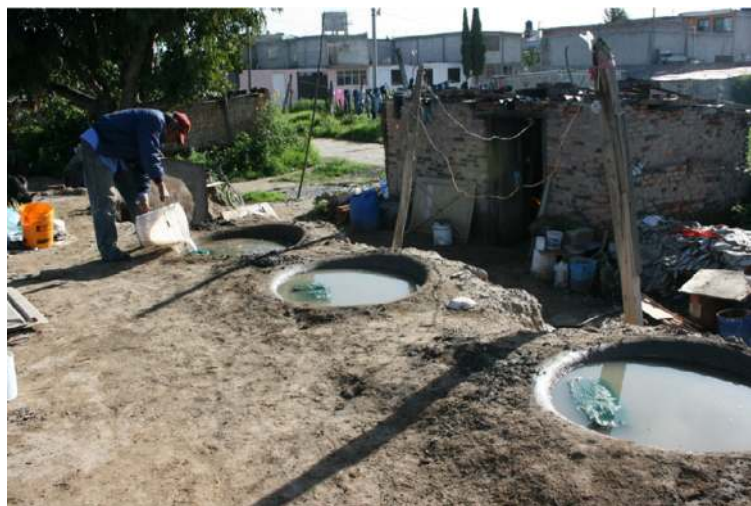
Figure 7. Nexquipayac, State of México. Pouring salt water in clay filters filled with salty soils during August 2008 (Photo by B. Castellón).
