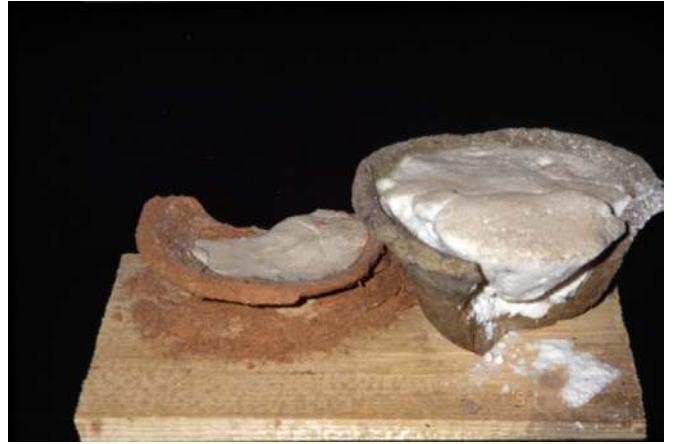
Figure 20. Stored salt a year later. The salt in the beveled rim bowl is in perfect condition, whereas the salt cake produced in an ordinary ceramic vessel has caused the ceramics to crumble.
