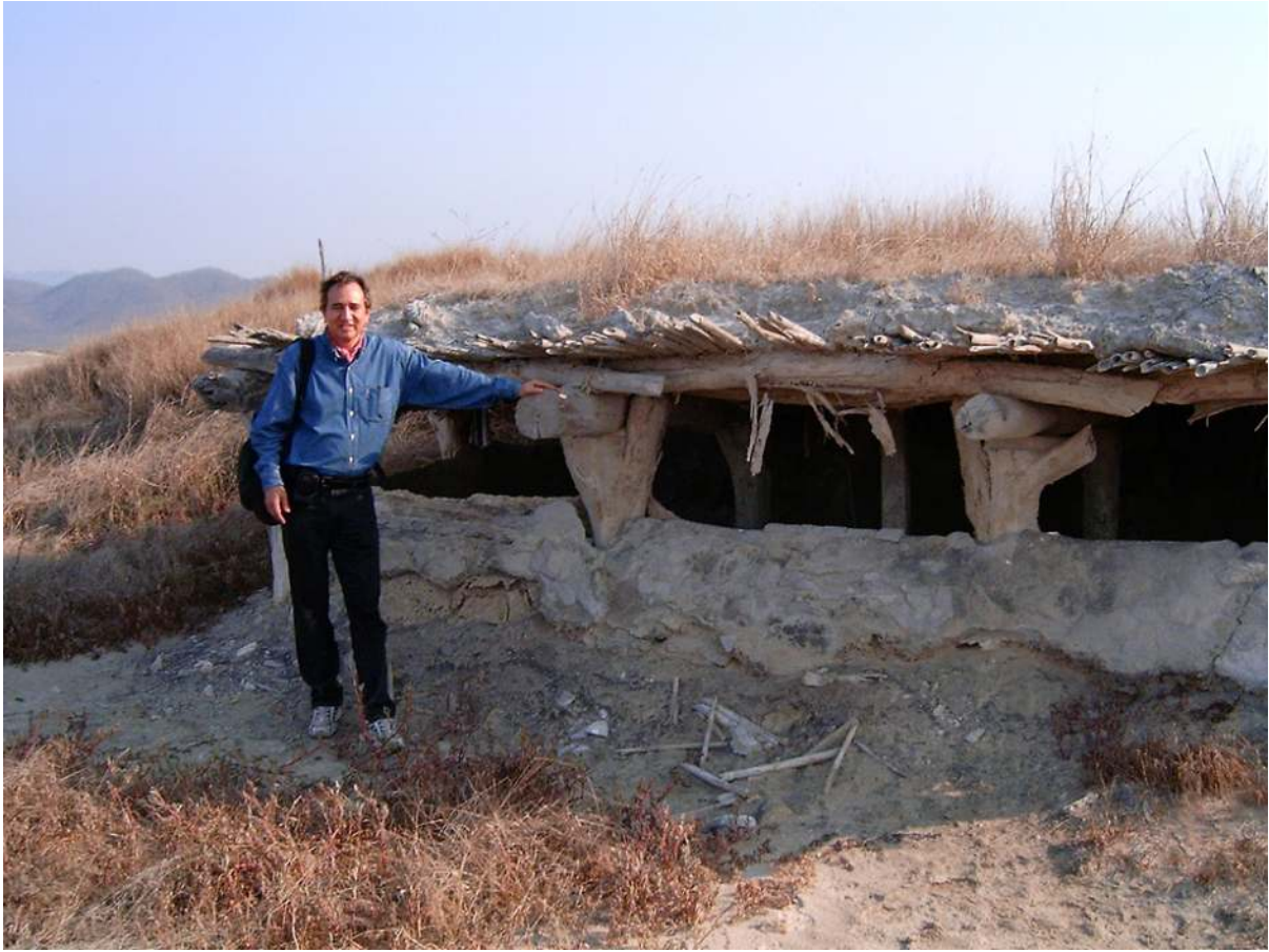
Figure 9. Lagoon of Cuyutlán, Colima. Large filtering mechanism abandoned in May 2006. The salty soils were loaded in the top and the water poured into the small room below (Photo by B. Castellón).
