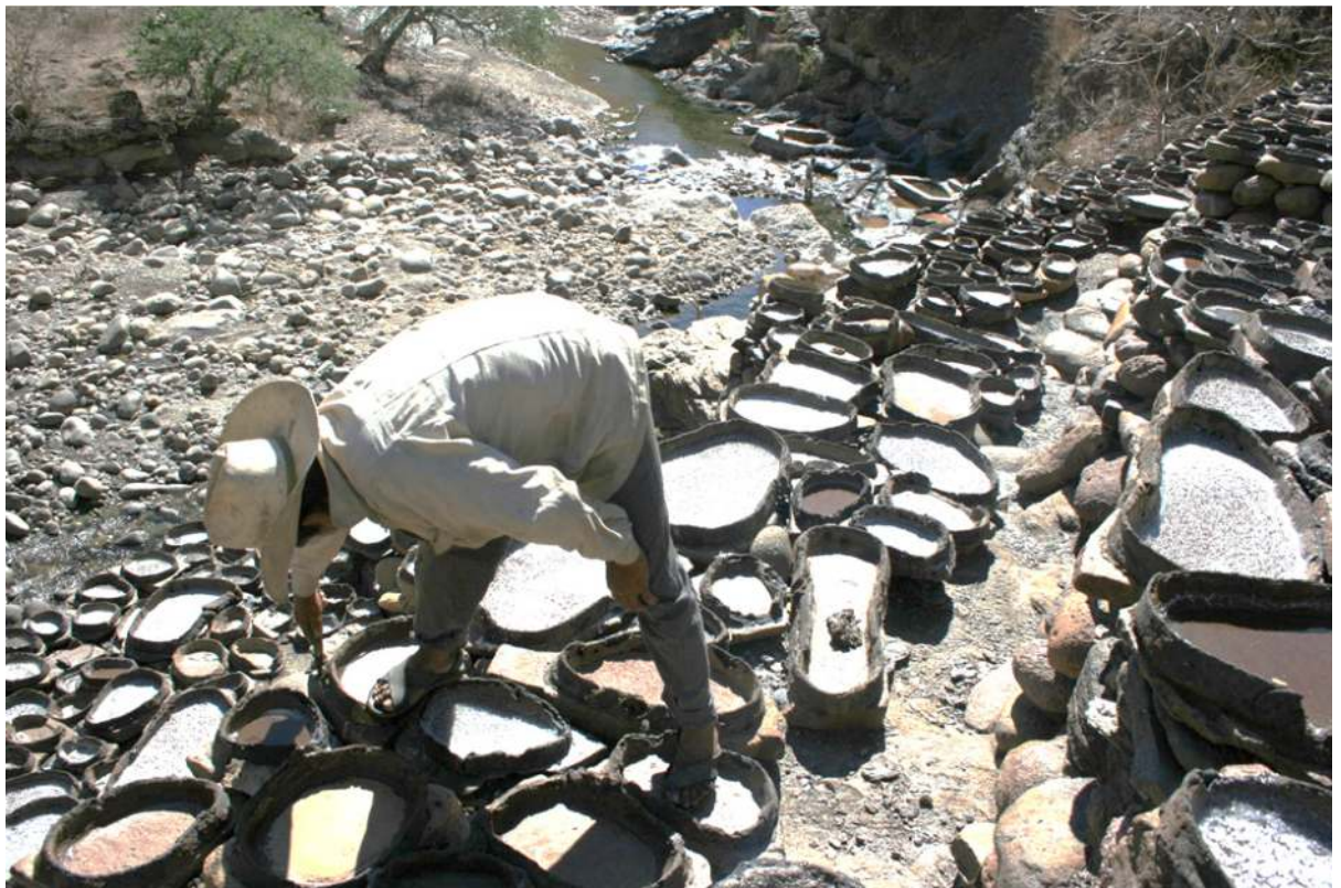
Figure 10. San Miguel Ixtapan, located in San Francisco, State of Mexico. Repair of poches or bowls where salt crystallizes, in May 2009 (Photo by B. Castellón).
