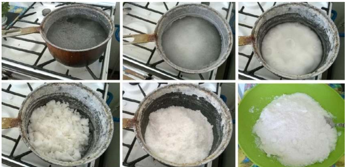
Figure 7. Making fine, white table salt by boiling the brine (experiment by F. A. Tencariu).
