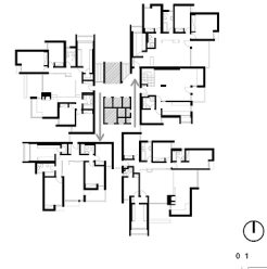
Figure 4. Plan of Alfragide Residential Complex: even floors plan; gray hatch highlights the utility core. Drawing by the authors.
