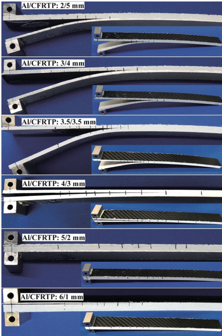
Fig. 72 Al/CFRTP thickness ratio dependence on the plastic deformation of the Al beams after the DCB test of the Al/CFRTP adhesive joints. The total thickness is fixed at 7 mm and the thickness ratio is varied. Reprinted with permission from [85]. Copyright 2020, American Chemical Society. All Rights Reserved
