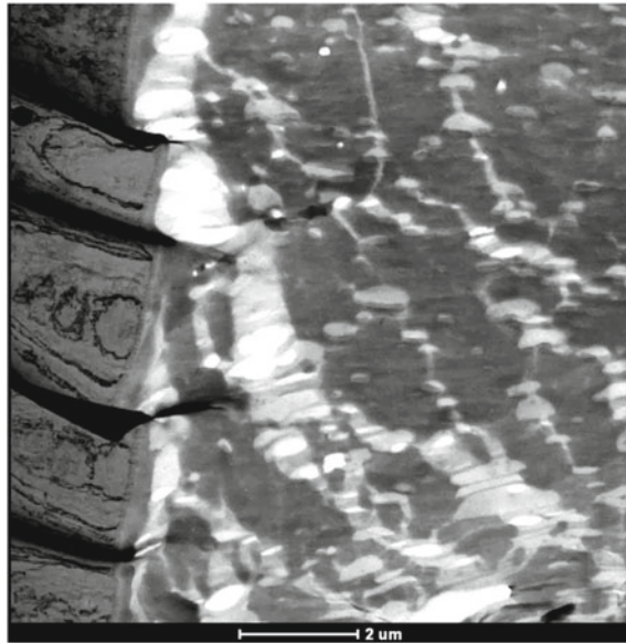
Fig. 64 Video showing the failure behavior of the PPS/Al direct joint in STEM bright-field (BF) mode
