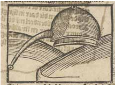
Fig. 3.1. Alembicum (detail of Fig. 3.14). Die distellacien ende virtuyten der wateren (Brussels: Thomas van der Noot, 1517), fols. a6v–b1r. Washington, D.C., Library of Congress, Rosenwald 1139. [Dist-1517-W02]
