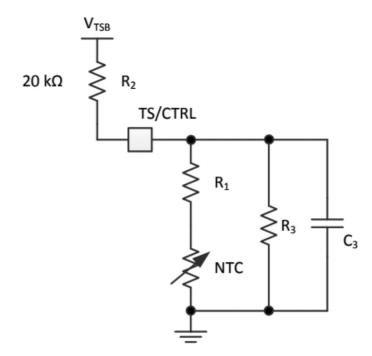
Figure 3.6 Circuit to control the battery's temperature. Source: Texas Instruments.
