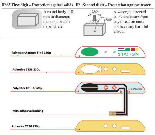
**Table 3.5** The IP code for STAT-ON<sup>™</sup> is IP65.
