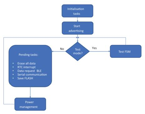
Figure 3.11 nRF firmware structure FSM.
