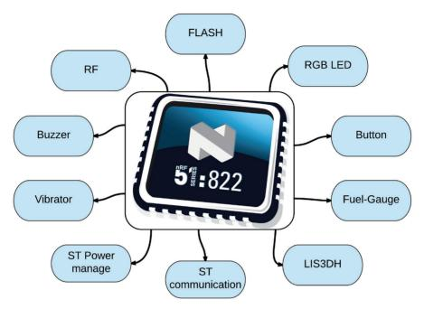
Figure 3.10 nRF51822 system with related modules.
