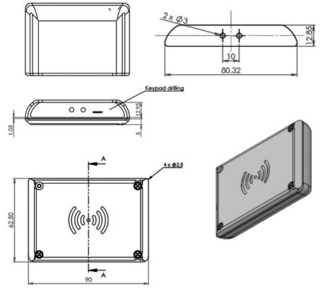
Figure 3.17 Housing overall dimensions.
