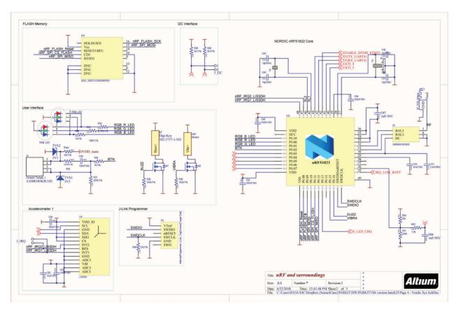
Figure 4.5 The schematics example corresponds to the nRF51822 processor.
