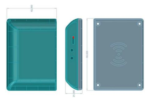
Figure 3.19 General measurements of the box.
