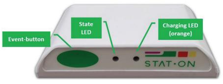
Figure 4.7 Sensor's interface.
