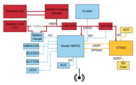
Figure 3.2 Sensor device architecture.
