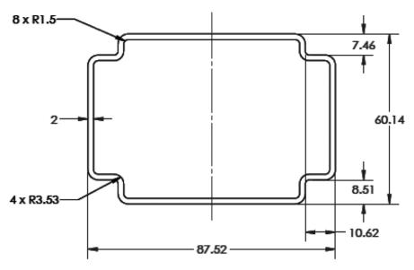
Figure 3.14 Sealing strip shape and dimensions.
