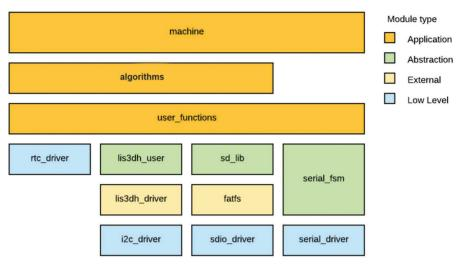
Figure 3.12 ST firmware code architecture.
