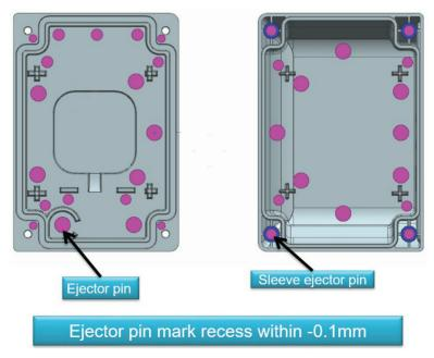
Figure 3.21 Ejection points.
