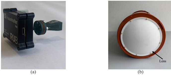
Figure 3.1: (a) The utilized radar sensor in high-resolution RCS measurement setup in this work. (b) The designed lens antenna which mounts on the radar and focuses its main beam for high-resolution measurements.
