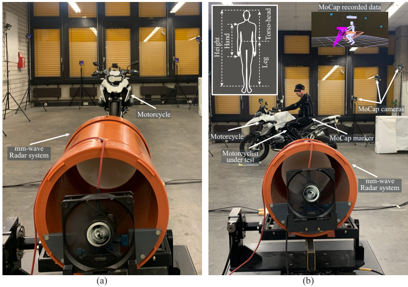
Figure 5.13: (a) Setup for measuring the clutter level of the test environment. The Radar system scans the test environment in the absence of a rider. (b) Setup for monostatic high-resolution RCS measurement to extract the range, velocity, and RCS information of different body parts of a motorcyclist in motion. The defined corresponding body parts (torso-head, hand, and leg) for measuring each body region are shown in the inset.
