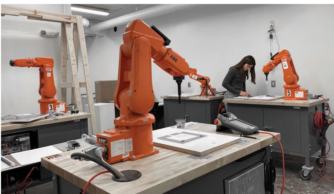
Figure 2. The tooling setup with five tabletop ABB robots equipped with 3D-printed pen holders.
