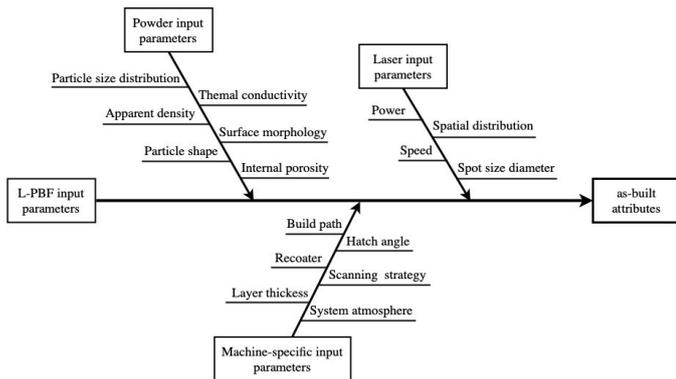
Figure 3. A schematic diagram showing a summary of L-PBF input parameters.
