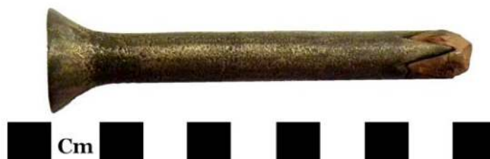
Figure 3. Possible rivet snap, British Museum (photo by author © Trustees of the British Museum)
