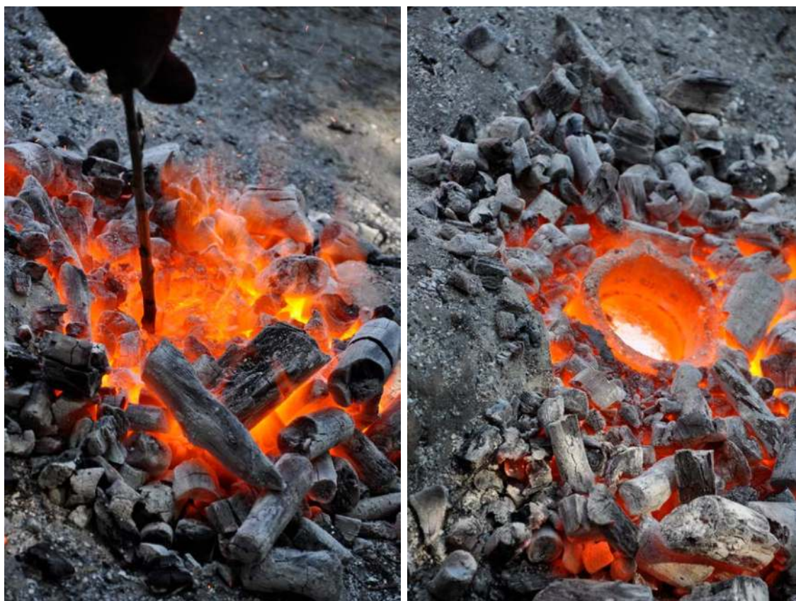
Figure 2. Four different moments of the casting process: a) the crucible is covered with charcoal; b) bronze has reached the melting point;
