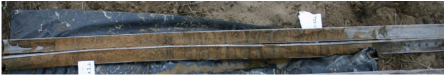
Fig. 16.3 Distribution of AC throughout aquifer sands after high-energy injection. The sleeve is a standard 3.6-cm diameter tube
