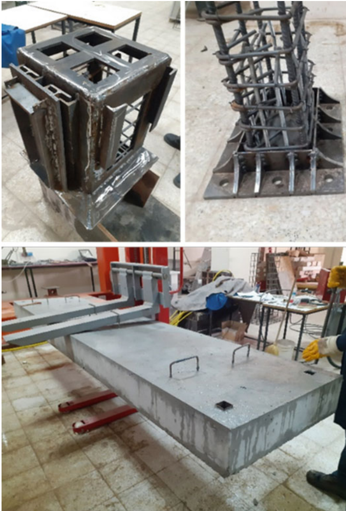
Fig. 14.3 Details of connections of demountable structural elements
