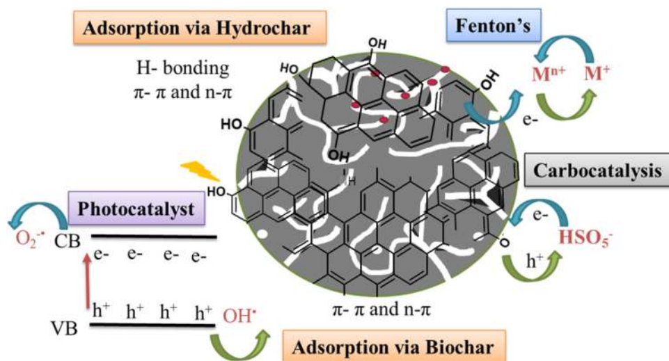
Figure 16.2 Schematics of sorption and degradation mechanism using waste-derived carbon materials and composite.
