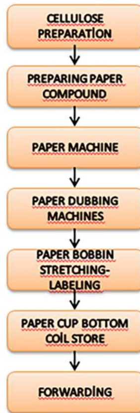
Figure 7.7 Pulp and paper manufacturing production processes.
