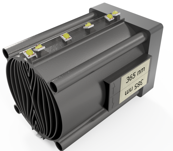
Figure 7.5: Rendering of a the CAD model of the LED light source modules shining their light into the optics module of the developed isophotonic photoreactor. The small inclined pillars on which the SMD LEDs are placed ensure the derived optimal inclination and positions of the LEDs resulting in an isophotonic reaction volume.
