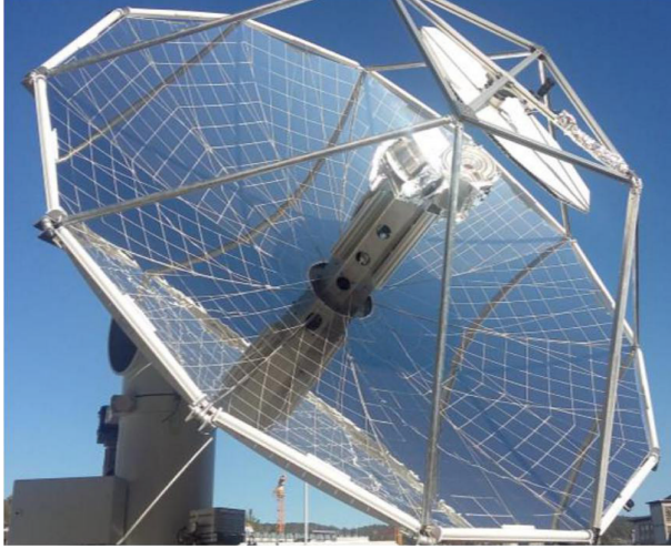
Figure 2.9: Highly concentrating photoreactor at the ETH Zürich employed to operate a solar-driven thermal catalyst system splitting carbon dioxide and water to yield synthesis gas in a high temperature redox cycle. Reprinted with permission from Springer Nature, [22], Copyright 2021.
