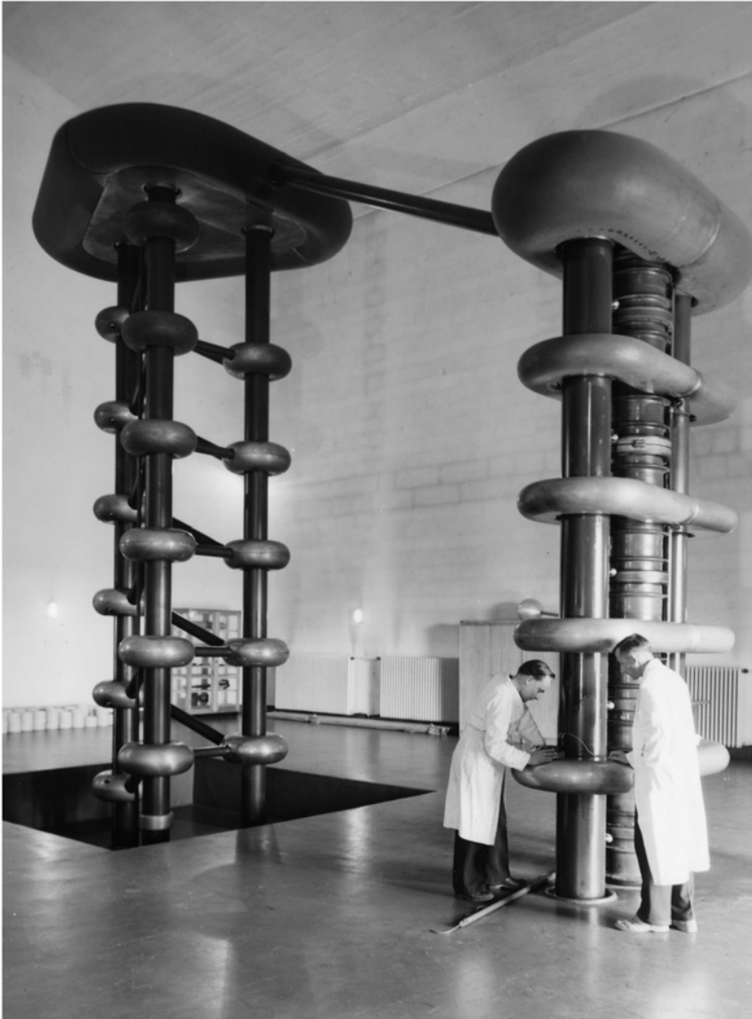
ILLUSTRATION 58 1.5 million-volt Cockcroft-Walton accelerator, Max Planck Institute for Chemistry, Mainz, June 6, 1956
