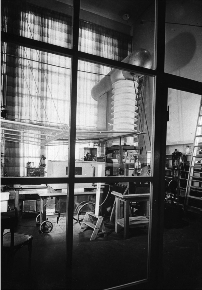
ILLUSTRATION 42 The Van de Graaff electrostatic generator at the Kaiser Wilhelm Institute for Medical Research in Heidelberg, 1936. This device, successfully employed by Bothe and Gentner for their experiments, accumulates electric charge, thereby creating very high potentials that can accelerate charged particles to high speeds, which in turn can be used to produce a variety of nuclear reactions. Such accelerators played a key role in the development of nuclear physics during the 1930s.
