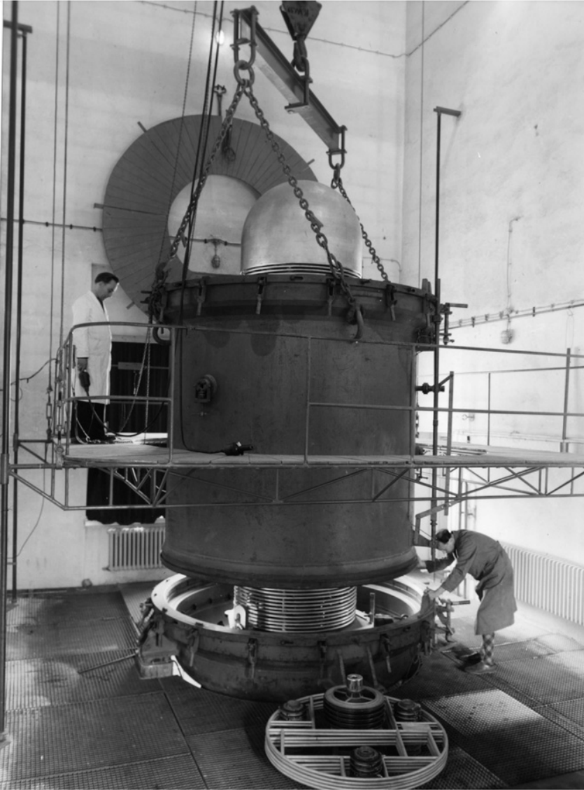
ILLUSTRATION 57 Van de Graaff generator for 3 up to 5 million volts. Max Planck Institute for Chemistry, Mainz, June 6, 1956
