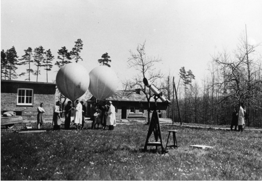
ILLUSTRATION 71 Research Center for Stratospheric Physics, Weissenau, early post-war years. Preparing the launch of a Regener's balloon tandem. The telescope was used to track the balloon tandem so that the payload could potentially be recovered intact before it touched the ground.
