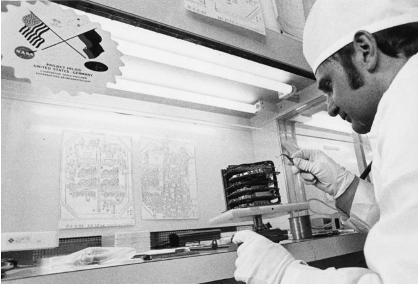
ILLUSTRATION 78 Max Planck Institute for Aeronomy, Lindau/Harz, assembly of parts of Experiment 8 of the Helios solar probe, around 1975
