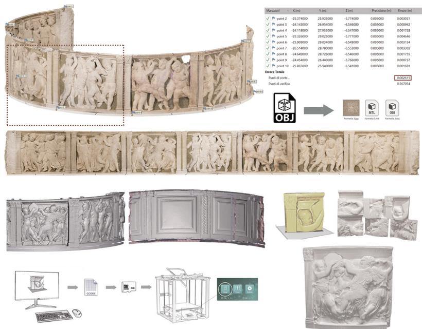
Fig. 7. Top: digital reconstruction of the tiles on a photogrammetric basis. Centre: orthorectified photoplane following projection of the cylindrical surface onto the plane. Bottom: model processing on AutoDesk Meshmixer software and images of a 1:1 scale 3D print of a tile. Graphic elaborations by the authors.
