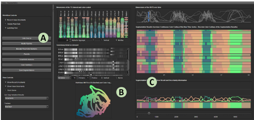
Fig. 6.6: Segmentation and labeling of radiation observations. (A) General segmentation workflow. (B) Data perspective including raw data, characteristics of individual variables, and dimensionality-reduced plot for patterns. (C) Overview and details of the multivariate time series and the segmentation results. © Courtesy of Jürgen Bernard.
