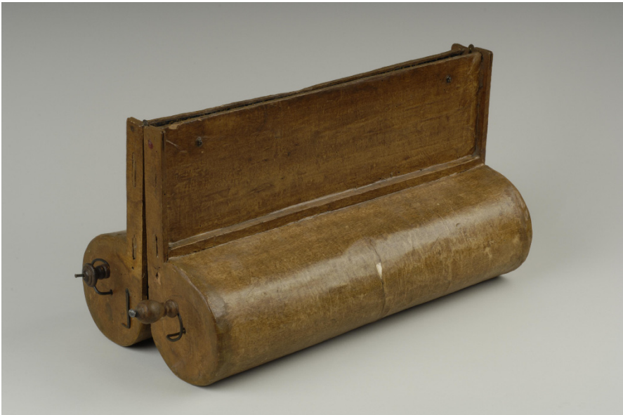
Fig. 2.10: Carte chronographique by Jacques Barbeu-Dubourg (1753) that shows the known history from the beginning of time up to 1760. Multiple sheets of paper were glued together and mounted in the chronology machine which allows to manually scroll back and forth in time using two handles. © Courtesy of Rare Book Division, Department of Rare Books and Special Collections, Princeton University Library, from Princeton University Library Catalog .
