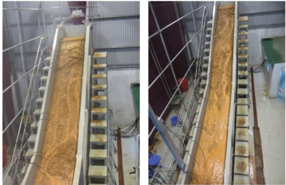
Fig. 26 The image of the Landslide experiment on a flume slope with artificial rains from the beginning stage and ending stage of the moving process
