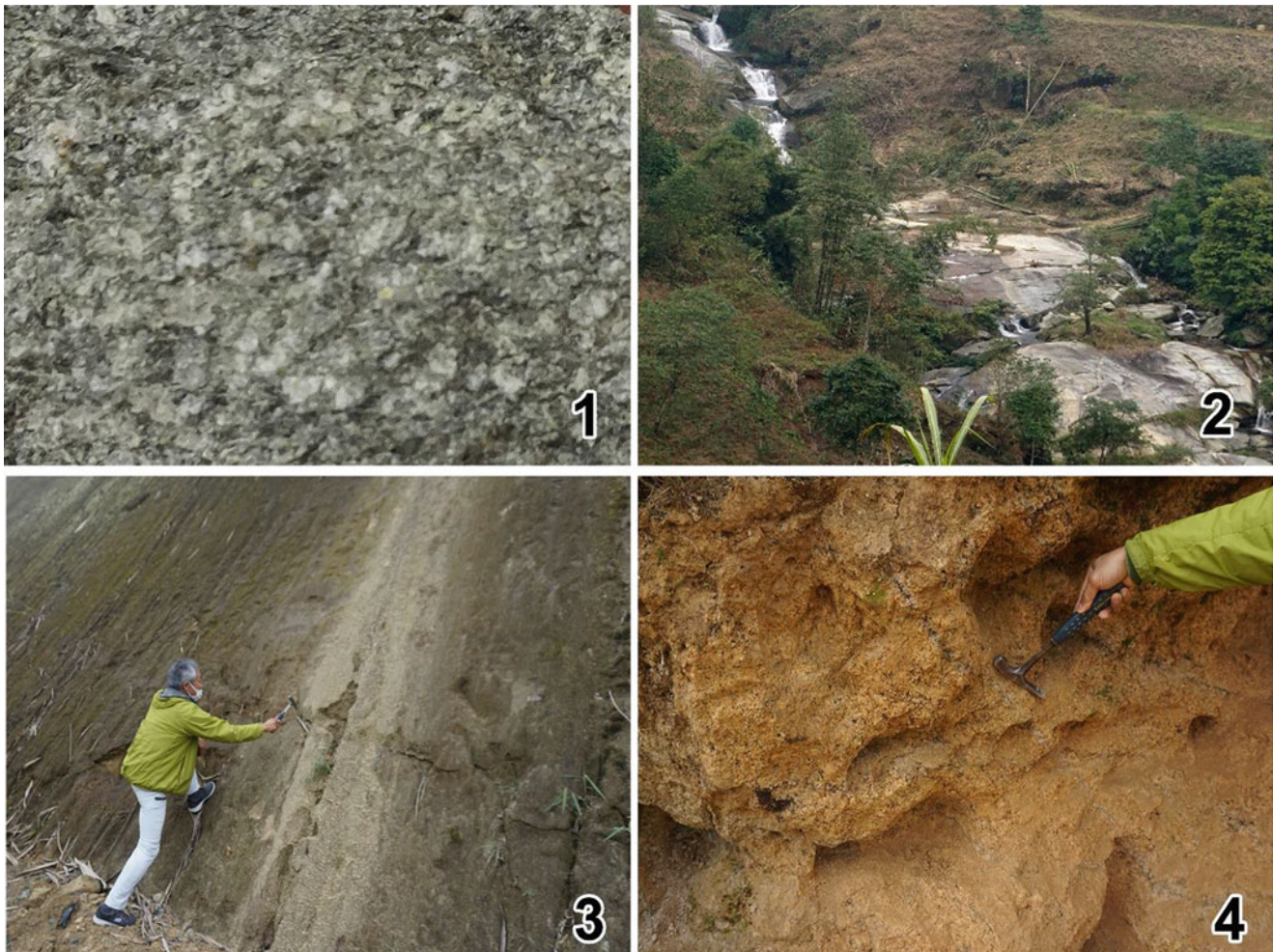
Fig. 5 Variety of the autochthonous rock facies compared with landslide materials at Trung Chai Commune, Lao Cai Province, Vietnam. (1) Fresh rock identified as “Granitic gneiss.” (2) Fresh hard rock facies
