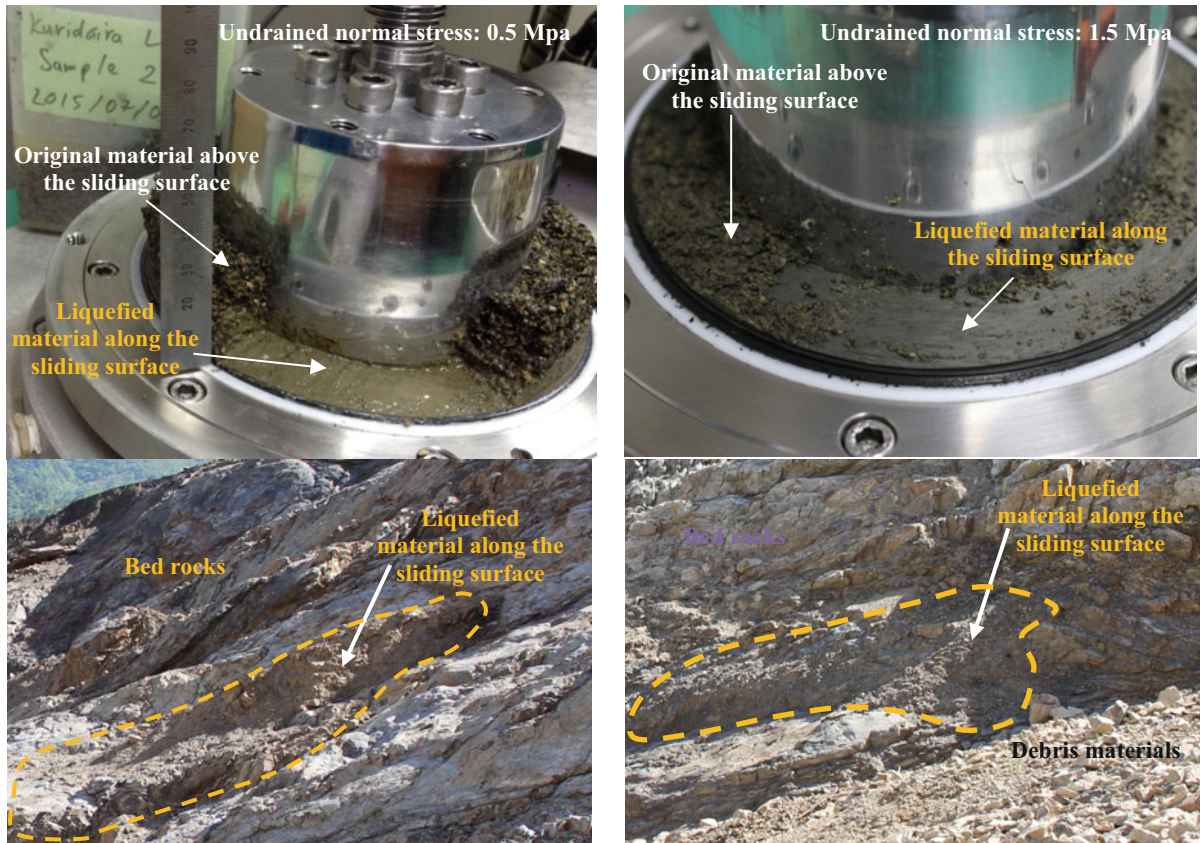
Fig. 84 Sliding surface liquefaction behavior of shale samples under different normal stresses in ring shear tests
