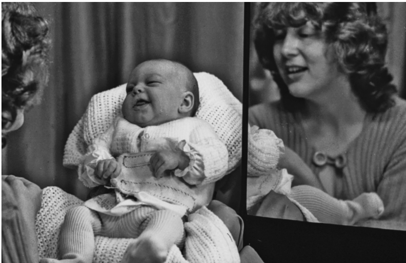
Figure 1.8 The 'en face' paradigm for recording infant–mother communication. The mother (her right shoulder and the side of her head is visible at left) has her image captured via a front-silvered mirror (on the right).
