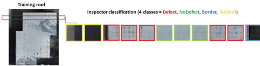
Fig. 8 Tiles representation of an examined roof associate to status classification
