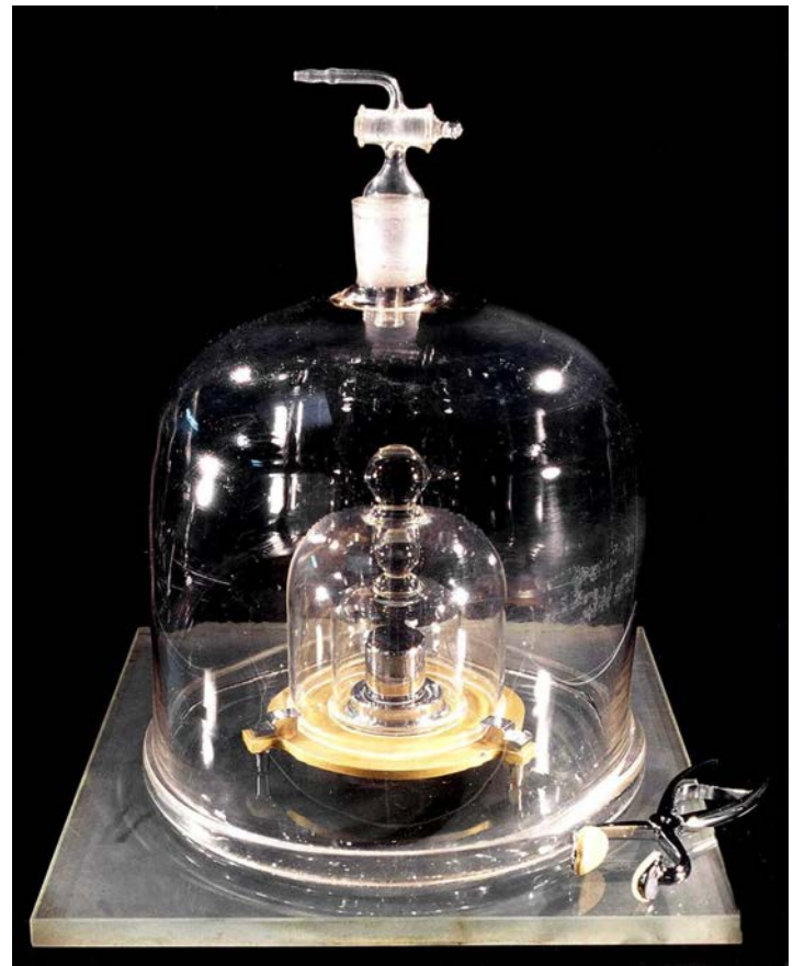
Figure I.3.1: The international prototype of the kilogram. Up to 2019, this was the standard of mass, kept under three glass bells in the Bureau International des Poids et Mesures in Paris. (Source: Wikimedia)
