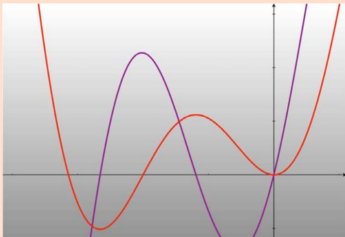
(a) The derivative df/dx (purple) of a function f(x) (red). At the extrema of y(x) the derivative (= slope) is zero.
