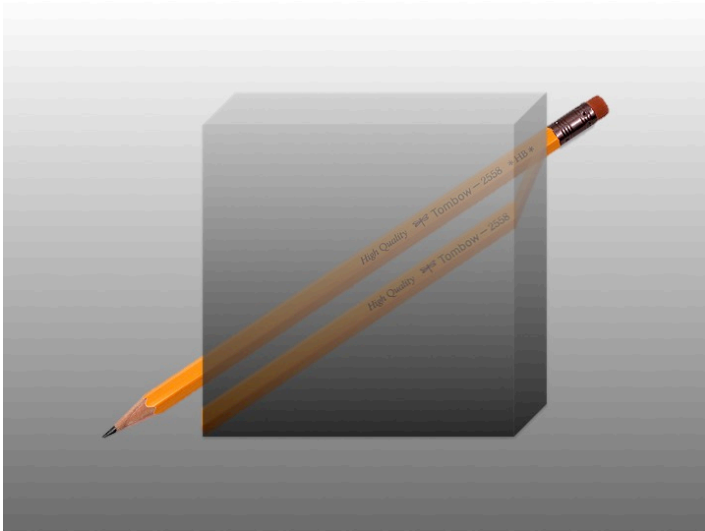
Figure II.3.10: Icelandic crystal . Double refraction of light by an Icelandic crystal or calcite.
