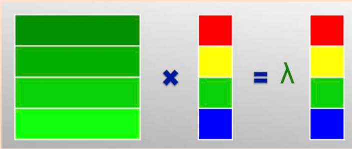
Figure A.9: Eigenvectors and eigenvalues . Given a matrix one defines the eigenvectors as a set of special vectors which satisfy an eigenvalue equation (A.8).
