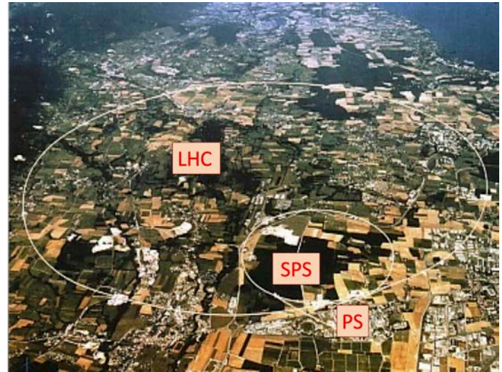
Figure I.4.42: The Large Hadron Collider at CERN . The largest accelerator at this moment is the Large Hadron Collider (LHC) at CERN in Geneva. The protons are accelerated in two oppositely directed circular beams. The circumference of the large ring is 27 km. Pre-acceleration happens in the older Proton Synchrotron (PS) and the Super Proton Synchrotron (SPS) accelerators.
