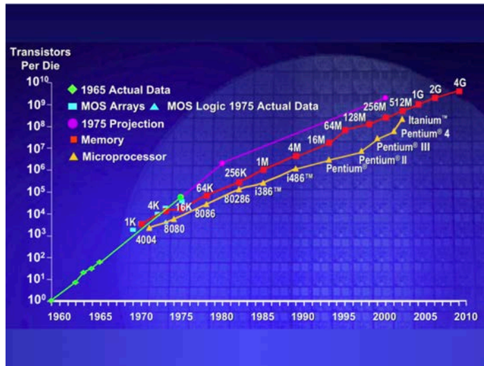
Figure I.2.48: Moore's law . This law states the astonishing fact that over the last half a century the power of computing has doubled every 18 months. The continuous downscaling of the basic components forces us to enter the gates of quantum domain. (Source: High Tech Forum)
