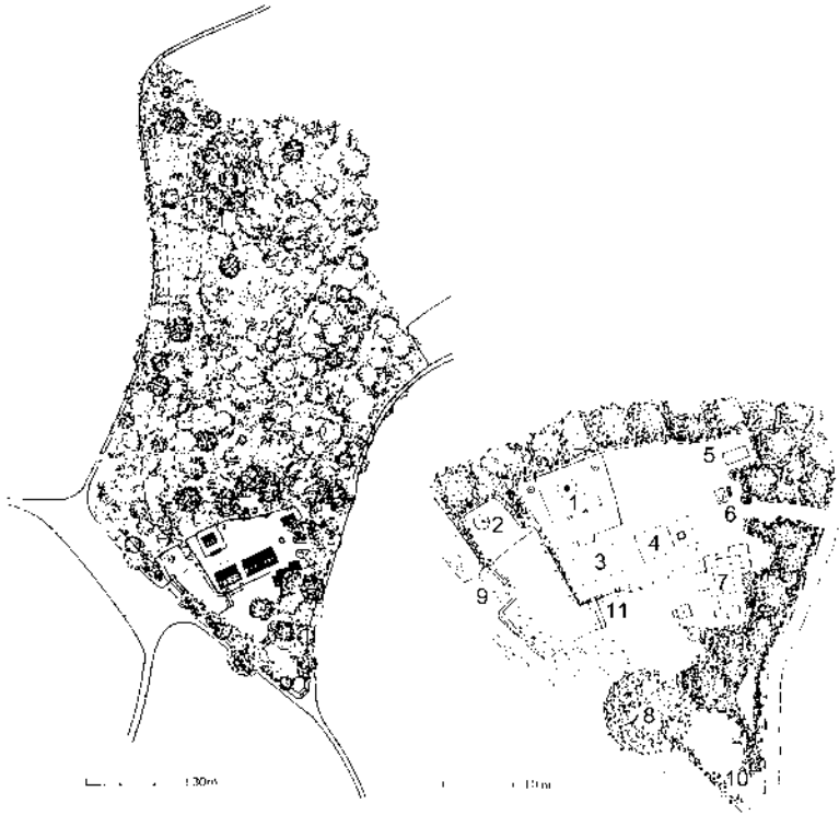
FIGURE 60 Plan of the Matsushita Jinja and plan of its public part (right). Ise shi, Futami-chō. (1) The main shrine or honden, raised on piles and enclosed by a fence; (2) The sanctuary dedicated to Somin Shōrai; (3) Haiden (prayer hall); (4) Okomori-dō (hall of confinement, used in a New Year's ritual); (5) Store-room; (6) Well; (7) Shamusho (shrine office); (8) An old camphor tree (prefectural natural monument); (9), (10) and (11) torii. Author's plans SOURCE: DOMENIG 1997: 94 (ADAPTED)
